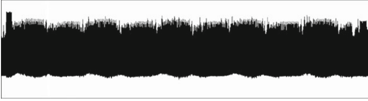
Fig. 1.4 Power consumption trace of a single AES encryption performed by a smart card
